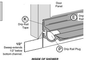
Drip rail may be additionally secured by drilling with 1/8" drill bit through drip rail into bottom channel. Attach using 8A x 3/8" truss head screws. When drilling in door panel, make sure drill does not hit glass. Glass is seated approximately 1/2" into channel.
